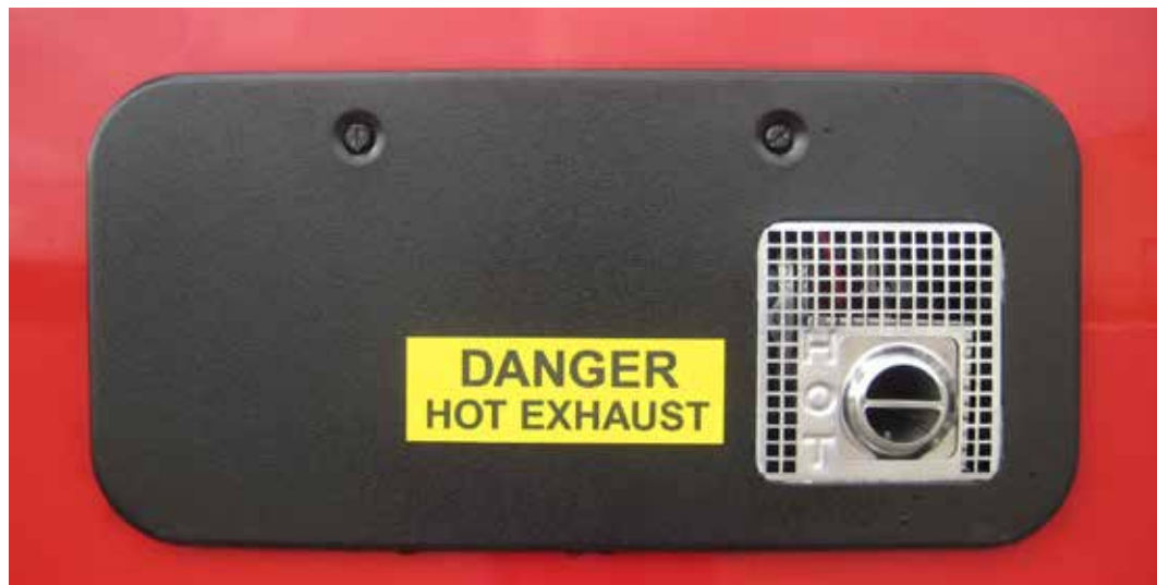
Furnace intake and exhaust on street side of trailer..
